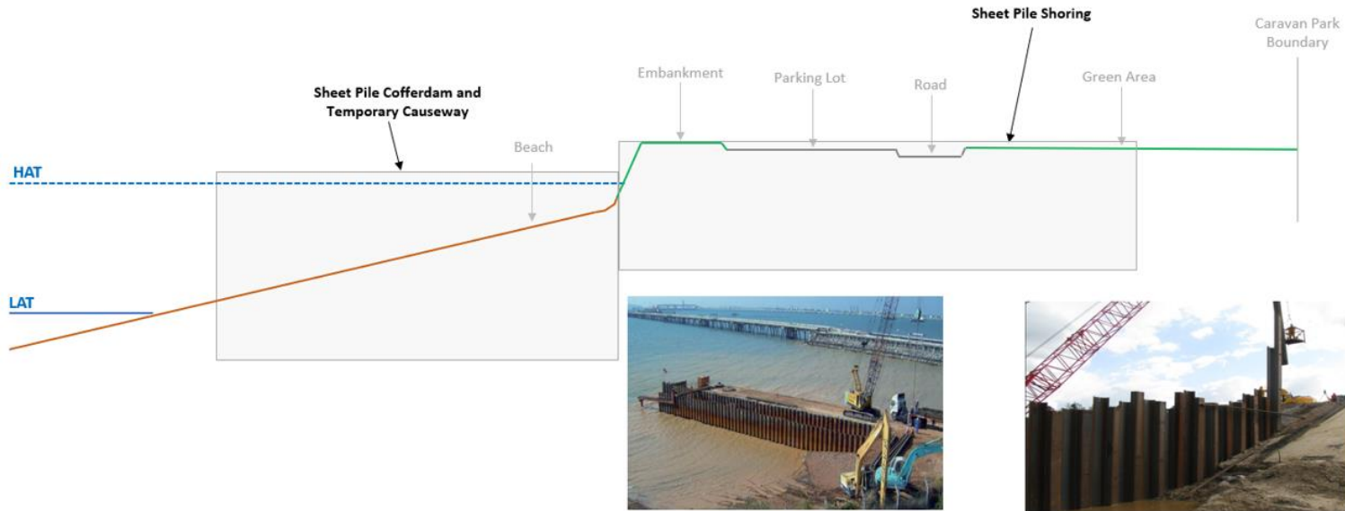
Figure 5.5 Temporary Works – Cofferdam and Causeway Construction
