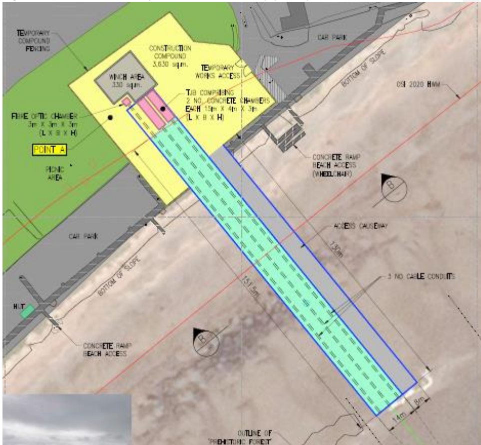
Figure 5.14 Construction/laydown Area Phase One (Option 1)
