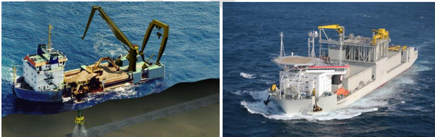
Figure 6.15 Typical Rock Placement Vessel
